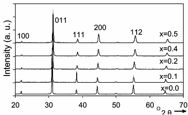
Figure 1. XRD pattern of  $\text{Ba}_{1-x}\text{Sr}_x\text{Ti}_{0.6}\text{Zr}_{0.4}\text{O}_3$  with different  $\text{Sr}(x)$  contents.
