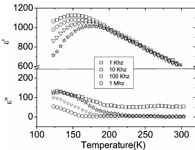
**Figure 3.** Temperature dependency of real and imaginary parts of permittivity of  $Ba_{0.5}Sr_{0.5}Ti_{0.6}Zr_{0.4}O_3$  at various frequencies.
