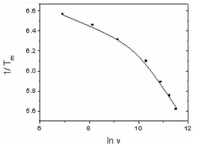
Figure 7. Plot of  $\ln(\nu)$  vs  $1/T_m$  as a function of the measured frequency of  $\text{Ba}_{0.5}\text{Sr}_{0.5}\text{Ti}_{0.6}\text{Zr}_{0.4}\text{O}_3$ . The symbols are the experimental points and line is corresponding fitting to the Vogel–Fulcher relationship.
