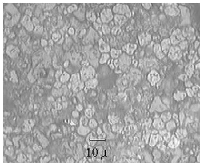
Figure 2. Microstructure of  $\text{Ba}_{0.5}\text{Sr}_{0.5}\text{Ti}_{0.6}\text{Zr}_{0.4}\text{O}_3$  ceramics.
