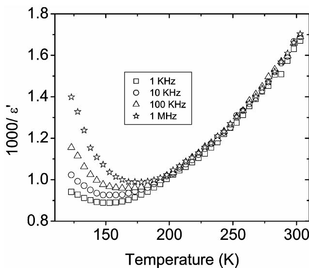
**Figure 4.** Plot of temperature dependency of  $1/\epsilon'$  for  $Ba_{0.5}Sr_{0.5}Ti_{0.6}Zr_{0.4}O_3$  at various frequencies.
