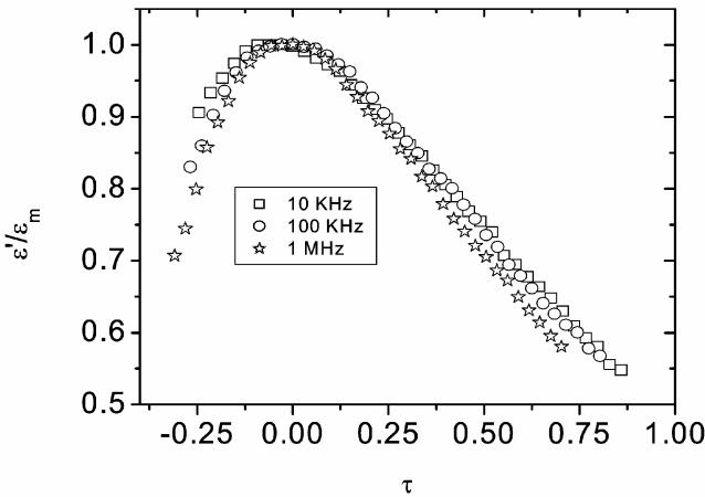
Figure 6. Plot of reduced dielectric constant,  $\varepsilon'/\varepsilon_{\max}$  vs reduced temperature,  $\tau$  [=  $(T - T_m)/T_m$ ] in the frequency range 10 kHz–1 MHz.
