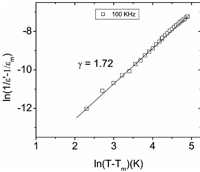
Figure 5. Plot of  $\log(1/\varepsilon' - 1/\varepsilon_m)$  vs  $\log(T - T_m)$  of  $\text{Ba}_{0.5}\text{Sr}_{0.5}\text{Ti}_{0.6}\text{Zr}_{0.4}\text{O}_3$  at 100 kHz.
