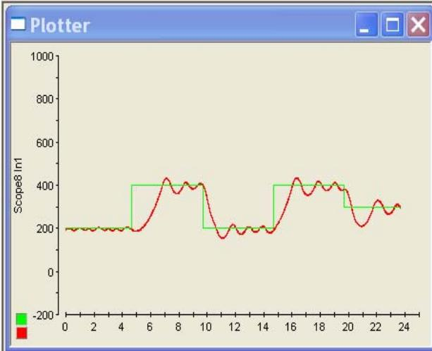
Figure 12. Experimental performance of actual speed versus change in command speed
