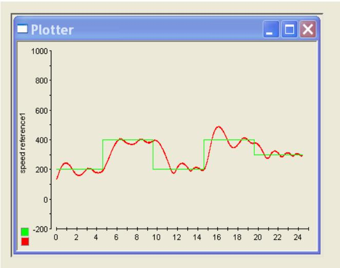
Figure 11. Experimental performance of PID vector control actual speed versus change in command speed
