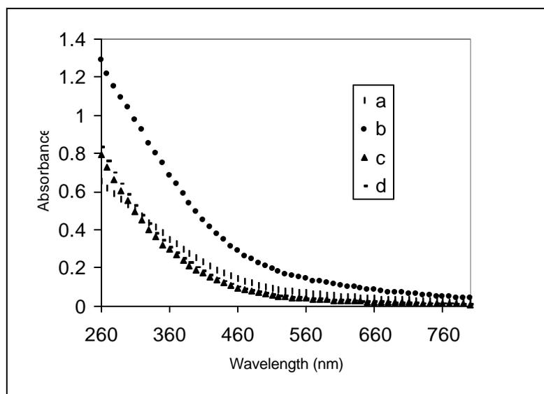
Figure 3. UV-VIS absorption spectra of CdS@Ag<sub>2</sub>S core-shell/composite nanoparticles prepared by (a) Post-core method, (b) Partial microemulsion (c) Simultaneous mixing, and (d) Pre-mixing method.
