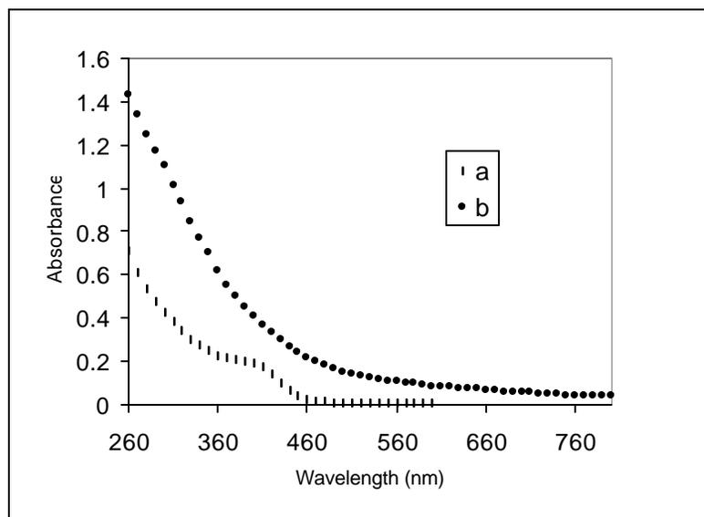
Figure 1. UV-VIS absorption spectra of (a) CdS and (b) Ag<sub>2</sub>S nanoparticles prepared in AOT/n-heptane / water microemulsion method at R=10.
