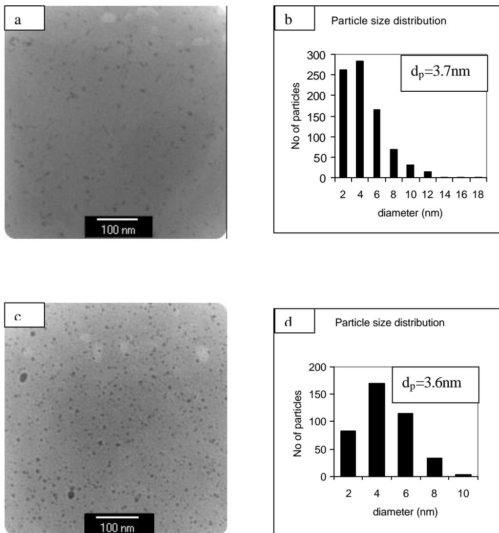
Figure 7. TEM micrographs and particle size distributions of CdS-Ag<sub>2</sub>S composite nanoparticles prepared by (a, b) Simultaneous mixing and (c, d) by Pre-mixing method.
