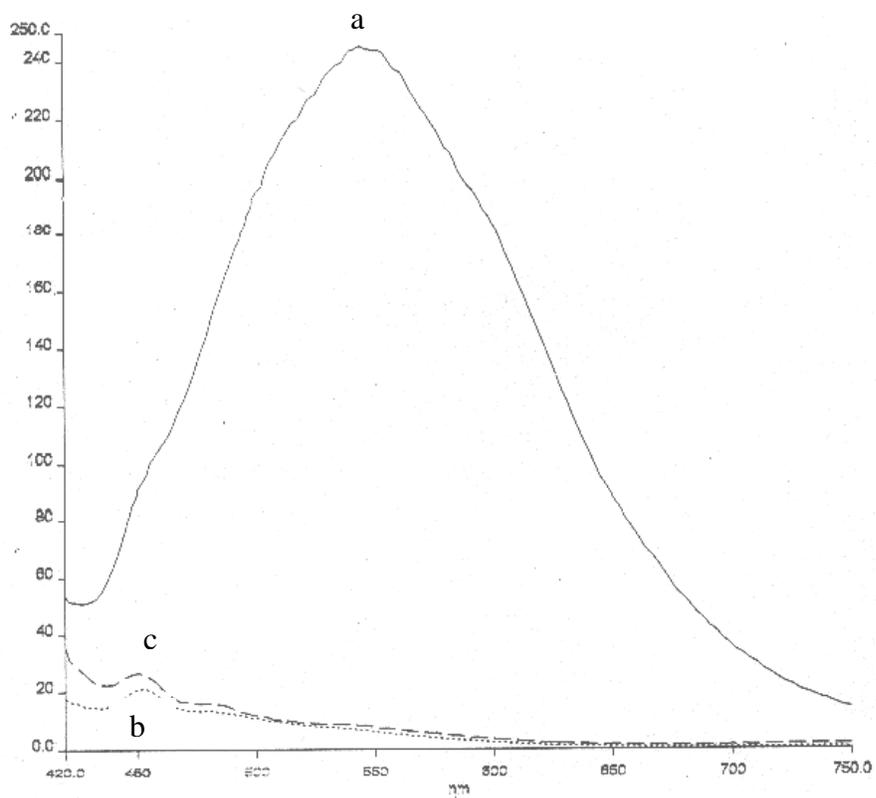
Figure 4. Fluorescence spectra of (a) CdS, (b) Ag<sub>2</sub>S and (c) CdS @ Ag<sub>2</sub>S nanoparticles prepared by w/o microemulsions at room temperature.
