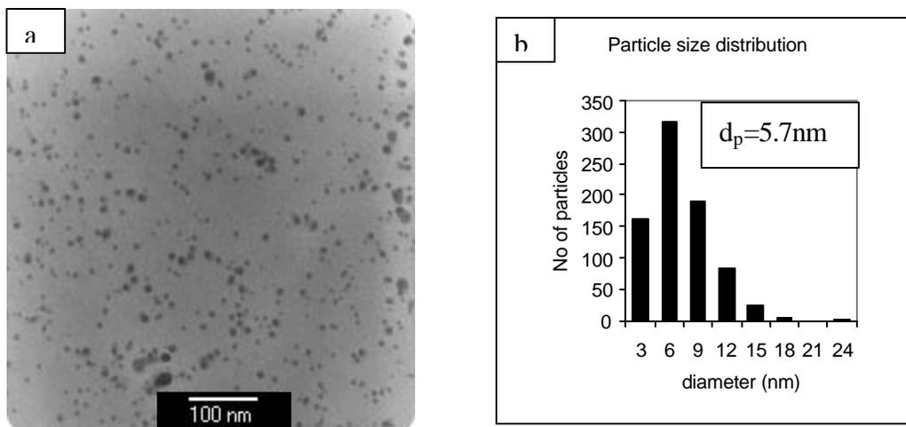
Figure 6. (a) TEM micrograph and (b) Particle size distribution of CdS @ Ag<sub>2</sub>S prepared by partial microemulsion method at R = 10.
