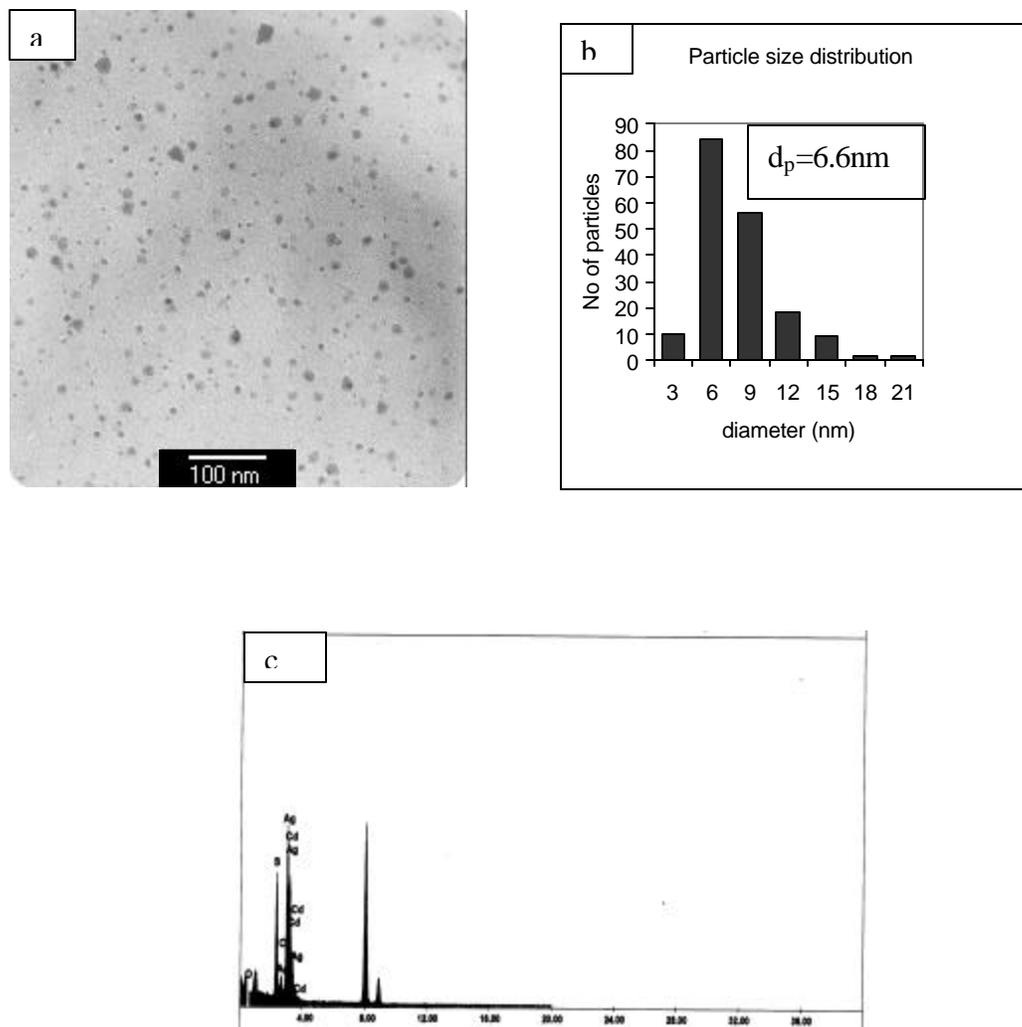
Figure 5. TEM micrograph, particle size distribution and EDAX of  $\text{Ag}_2\text{S}$  coated CdS nanoparticles prepared by post-core method using w/o microemulsions at  $R = 10$ .
