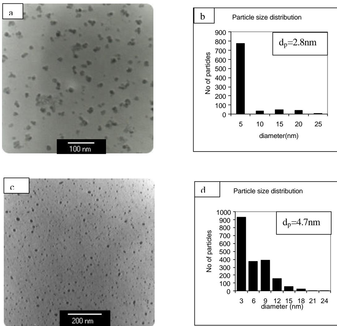
Figure 2. TEM micrographs, and particle size distributions of (a, b) CdS nanoparticles and (c, d) Ag<sub>2</sub>S nanoparticles, prepared in w/o microemulsions at  $R = 10$ .
