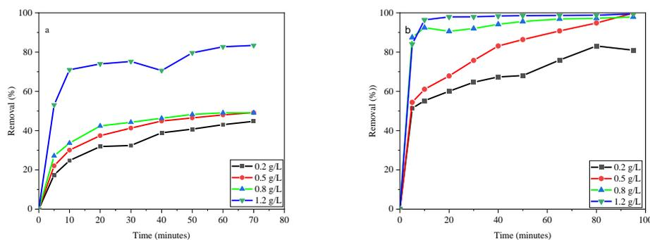
Figure 4: (a) Adsorption for Fe/MnBC dose variation (RhB = 3 mL, D.W = 27 mL, PMS = 0.0092 g). (b) Degradation with Fe/MnBC dose variation (RhB = 10 mg/L, catalyst = 1 g/L, PMS = 0.5 mmol).
