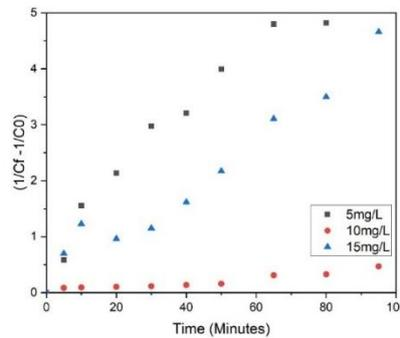
Figure 7: Linear second order Kinetics graph (Initial concentration: 10mg/L).
