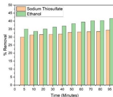
Figure 8: Effect of various radical scavengers' effect on removal of RhB (sodium thiosulfate=0.0047g, RhB=3ml, D. W=27ml).
