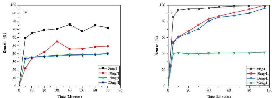
Figure 3: (a) Adsorption for RhB concentration variation: PMS = 0.009g, FeMn/BC = 0.015g. (b) RhB degradation with different materials (initial conc.=10 mg/L; catalyst dose =1 g/L; PMS = 0.5 mmol).
