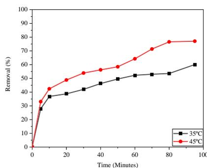
Figure 5: Effect of Temperature on Dye Removal Efficiency Using FeMn/Biochar Catalyst.
