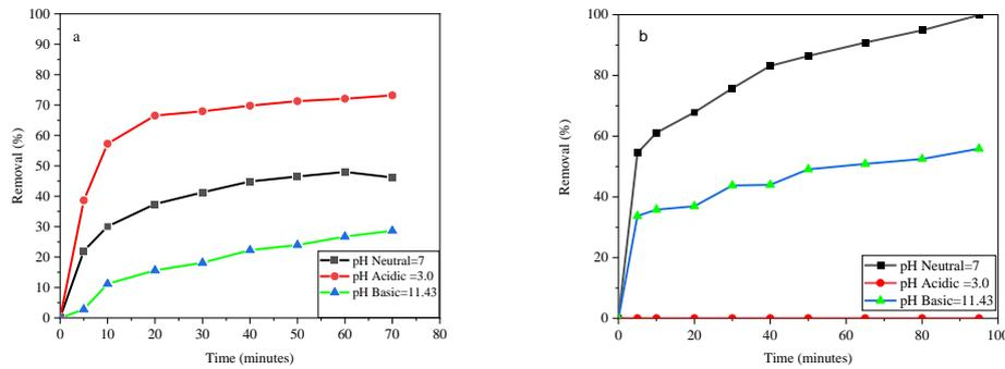
Figure 6: PH variation for (a)Adsorption and (b)degradation Graph for Fe/MnBC (0.015g), PMS (0.009g), D.W (27ml), RhB (3ml).
