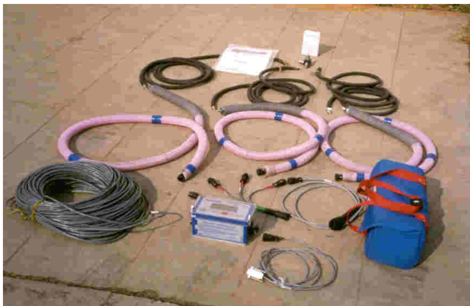
Fig. 2- Accelerometer based seismograph with accessories, Instantel Make
