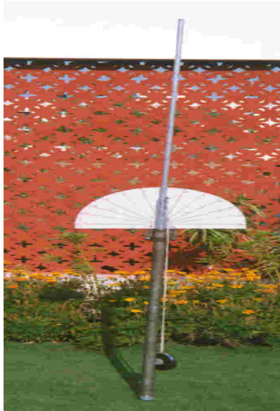
Fig. 3- Overbreak measuring telescopic rod, designed and fabricated in ISM, Dhanbad
