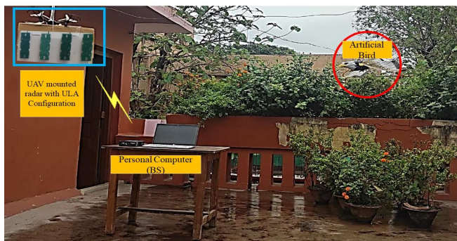
Fig. 2: Experimental set up for Artificial Bird with ULA arrangement
