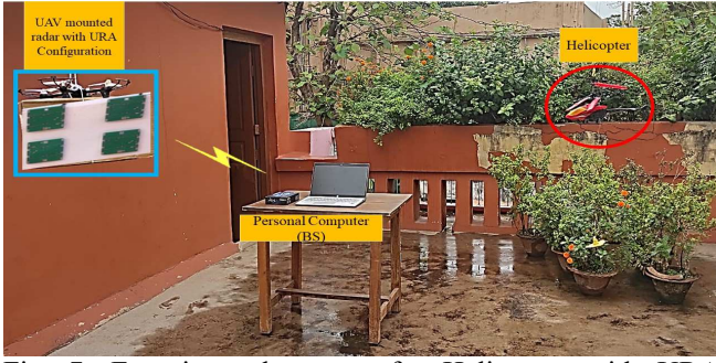
Fig. 7: Experimental set up for Helicopter with URA arrangement
