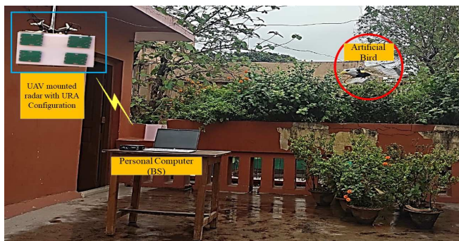
Fig. 3: Experimental set up for Artificial Bird with URA arrangement
