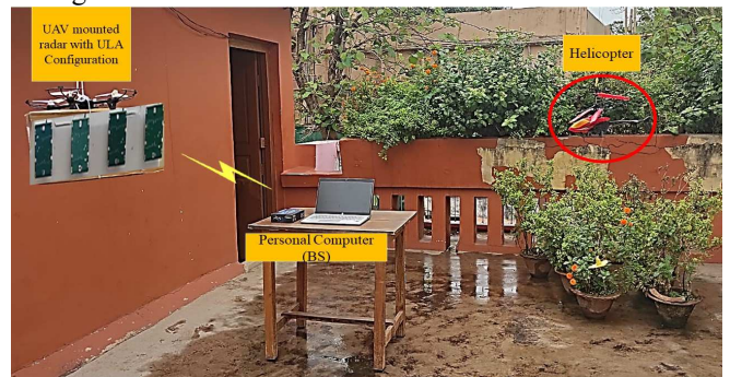
Fig. 6: Experimental set up for Helicopter with ULA arrangement
