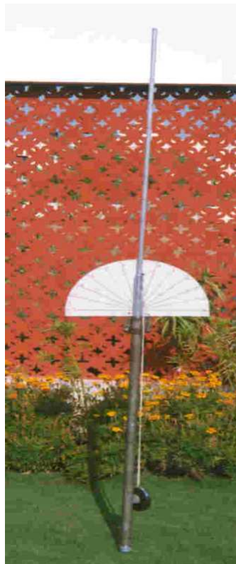
Fig 2: Overbreak measuring telescopic rod, designed and fabricated in ISM, Dhanbad
