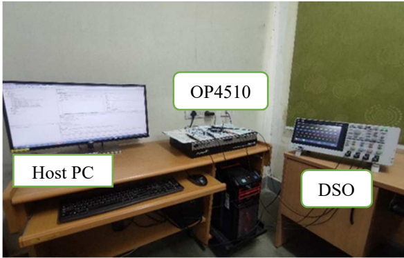
Fig. 13. Real-time experimental set-up using OPAL-RT.
