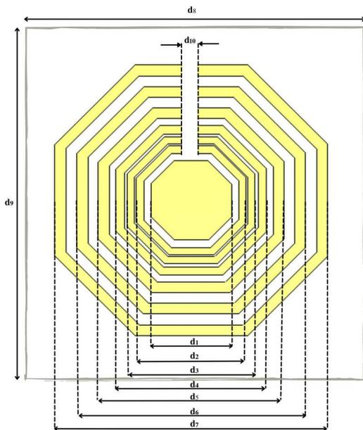
Fig. 2. Structure of transponder 1.
