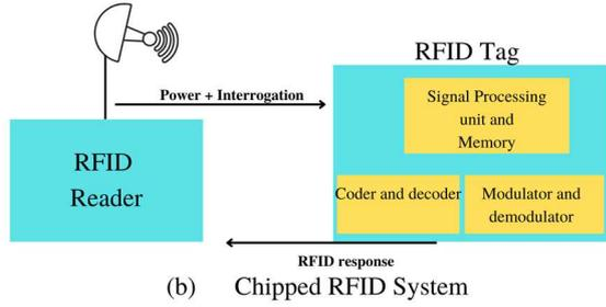
RFID system design. The structure of two transponders are discussed in sections IV and V. A comparative analysis is discussed in section VI. Finally, Section VII presents the conclusion with references at the end.
