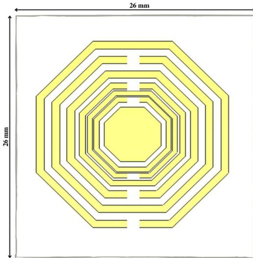
Fig. 5. Structure of transponder 2.
