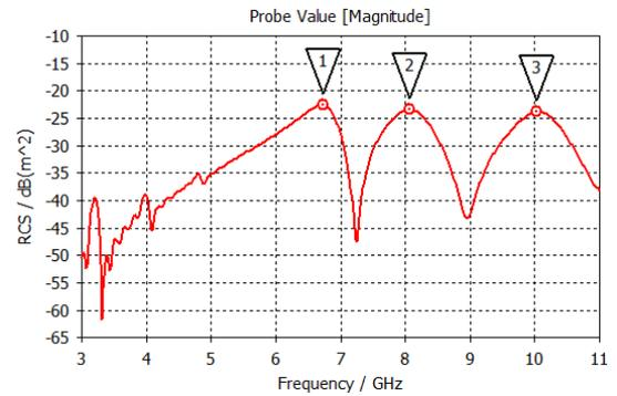
Fig. 3. RCS response curve of transponder 1.
