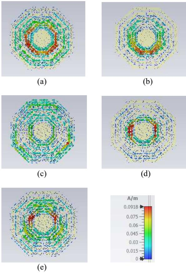
Fig. 7. Current distribution for transponder 2 at (a) 3.60 GHz, (b) 4.80 GHz, (c) 6.59 GHz, (d) 8.52 GHz, and (e) 10.25 GHz.
