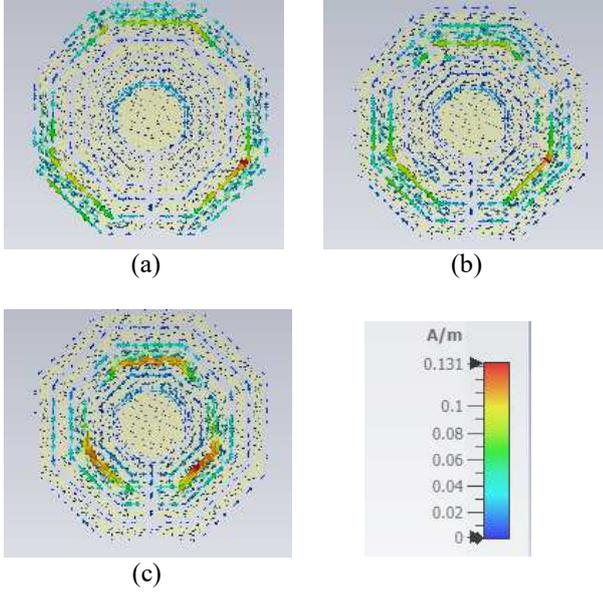
Fig. 4. Current distribution for transponder 1 at (a) 6.72 GHz, (b) 8.07 GHz, and (c) 10.04 GHz.
