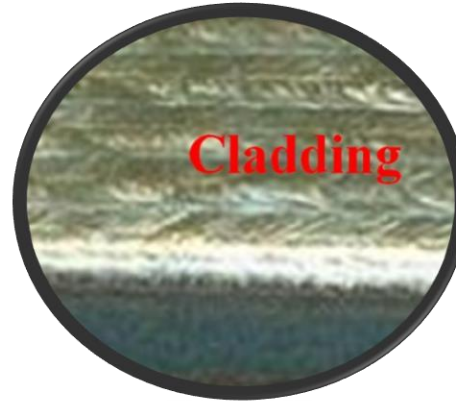
Side view of the morphology of laser cladding in grade 6 Stellite on carbon steel
