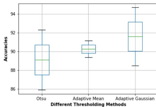
**Fig. 3** Box plot of the accuracies for the different thresholding methods
