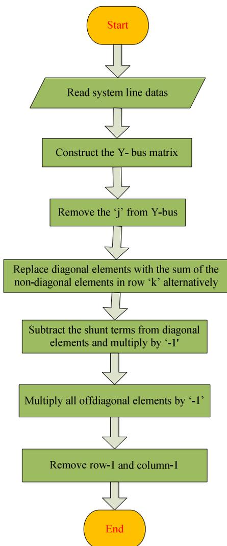
Fig.1: Flowchart for B' matrix construction
