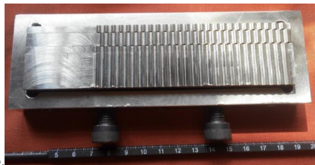
Figure 6: Fabricated rigid dies for the generation I and II bump foil a. Top b. Bottom
