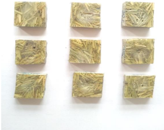
Figure 1: Samples (20*20*20 mm 3 ) cut from fabricated composite slab of size 150*5*60 mm 3
