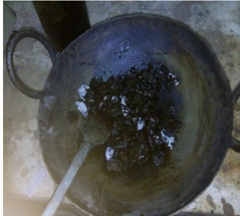
Fig. 1. Pretreatment of RCA using emulsion-water solutions
