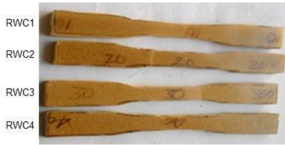
Fig. 3. Samples of Tensile test
