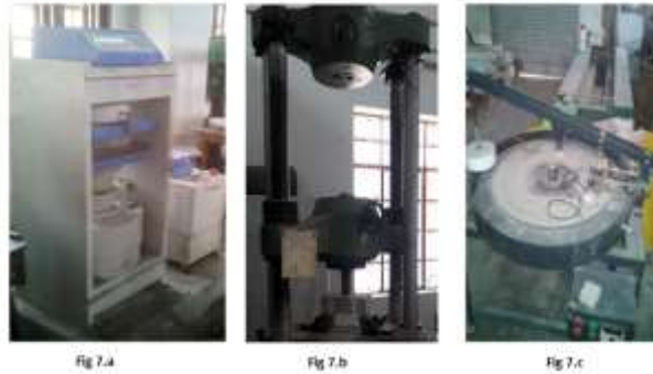
Fig.7. Test Set up for Compressive, Flexural Strength & Abrasion Resistance
