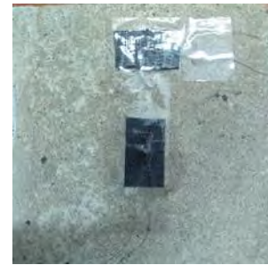
Fig. 2 Strain gauge installed on a specimen
