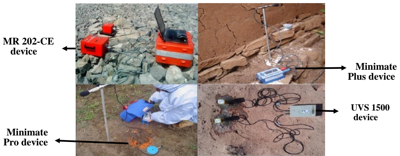
Figure 1. Various types of seismographs installed in mines
