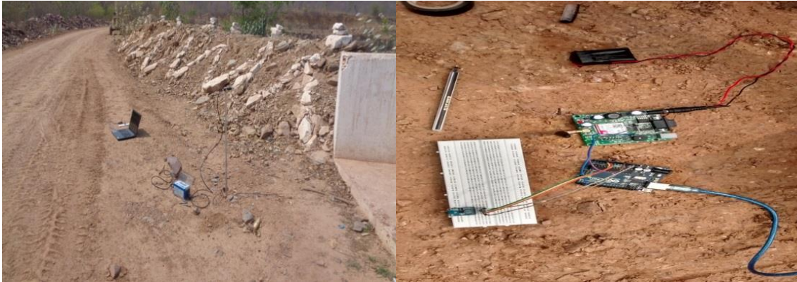
Figure 6. Installation of test bed in Mine-A
