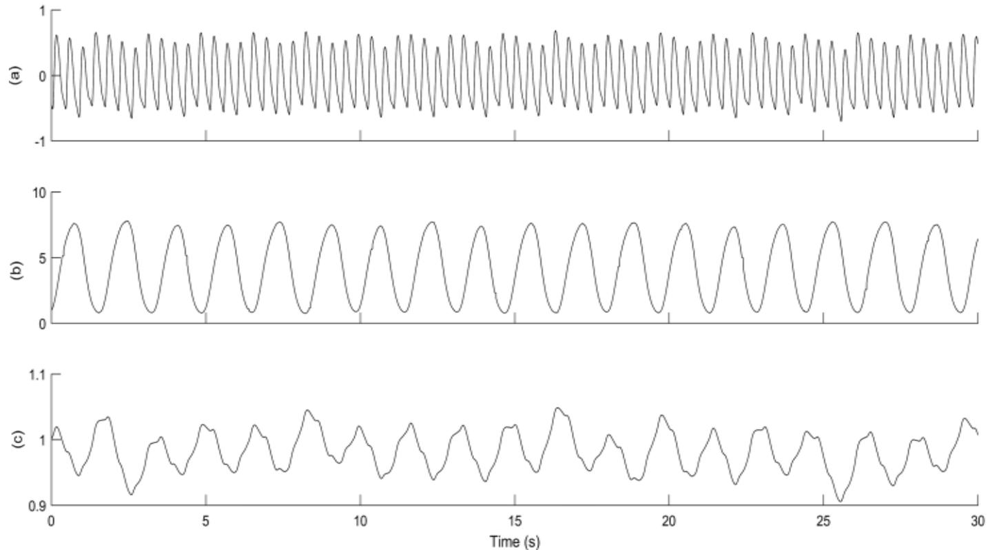
Figure: (a) PPG; (b) Reference respiration; (c) Largest component of PPG  $x_1(t)$
