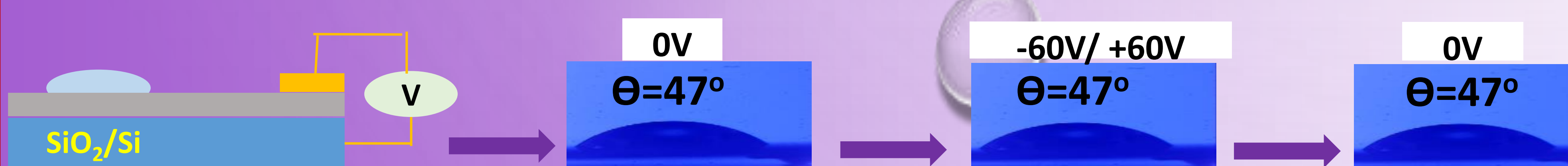
Wettability measurement on SiO_2 /Si surface at different voltages (-60 V/0 V/+60 V)
