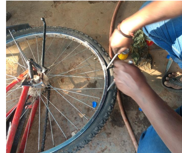
Fig. 3: Dismounting of bicycle tire
