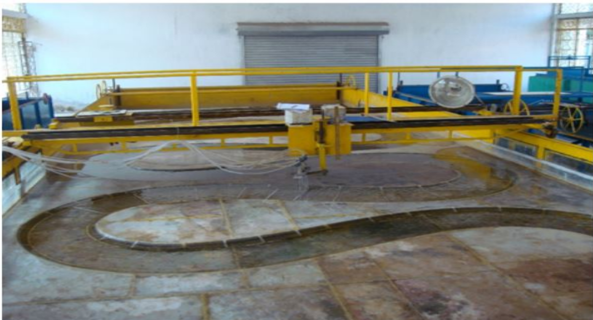
Figure 3 Meandering channel setup photograph
