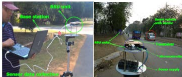
Figure-5 Experimental set up of RSU and base station in Rourkela city
