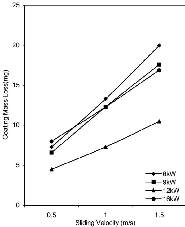
Fig.3 Variation in Wear Loss with Sliding Velocity
