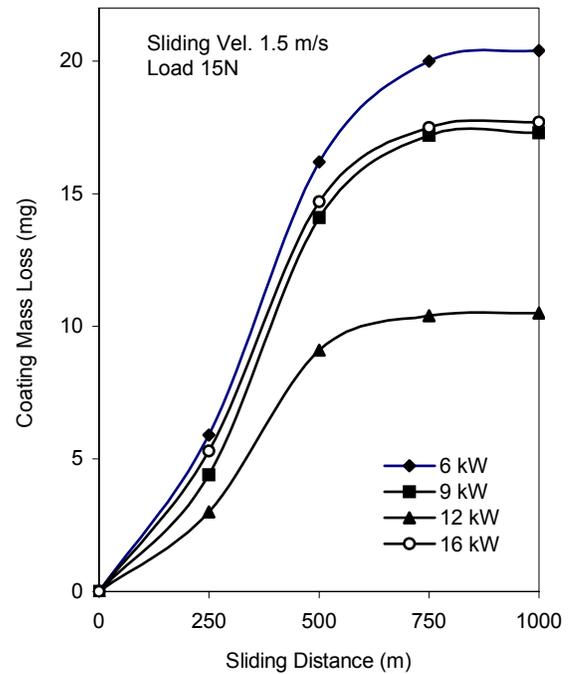
Fig. 2(c) Coating Wear (Mass Loss) Vs. Sliding Distance at velocity 1.5 m/s
