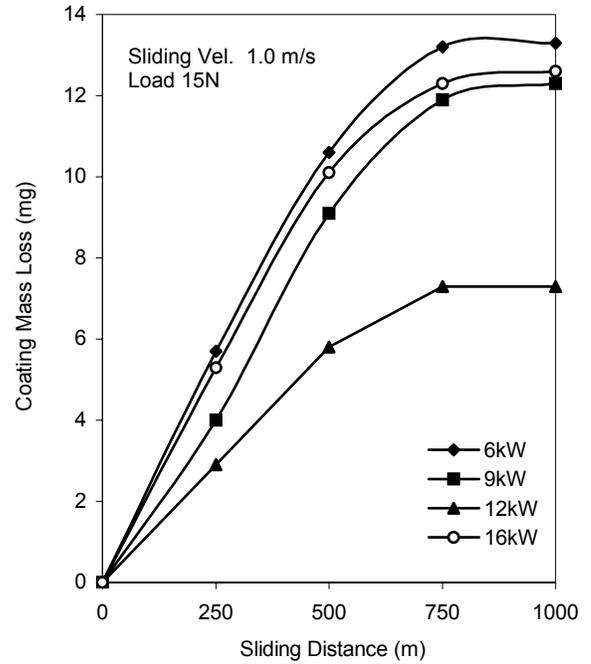
Fig. 2(b) Coating Wear (Mass Loss) Vs. Sliding Distance at velocity 1.0 m/s
