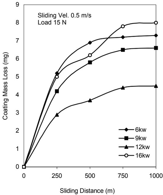
Fig.2 (a) Coating Wear (mass loss) Vs. Sliding Distance at velocity 0.5 m/s.
