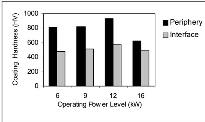
Fig. 1. Coating Hardness at Different Operating Power
