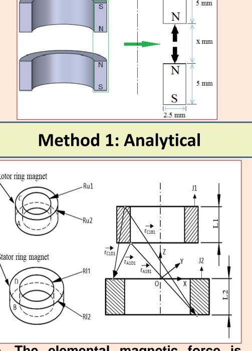
The elemental magnetic force is expressed in below Equation [2]. Where J and S are the magnetic polarization of the rings and surface area respectively. The elemental forces between elements of surfaces A-D, C-B, and C-D is calculated using the similar notations.
