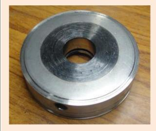
**Direct contact** between rotor and bearings during start and stop of the machine.
