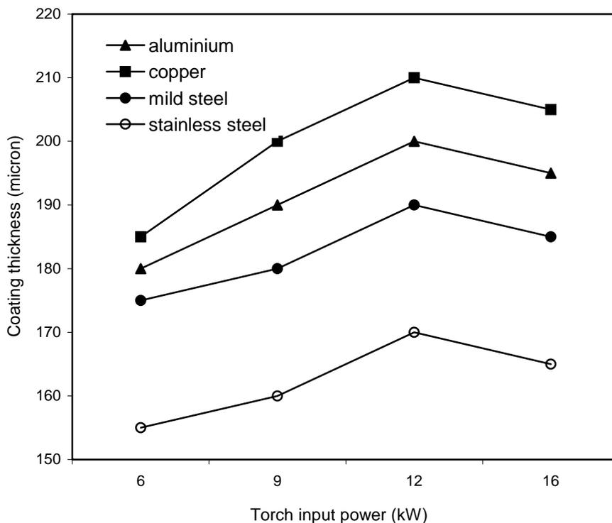
Figure 1 Thickness of red mud coatings made at different power level
