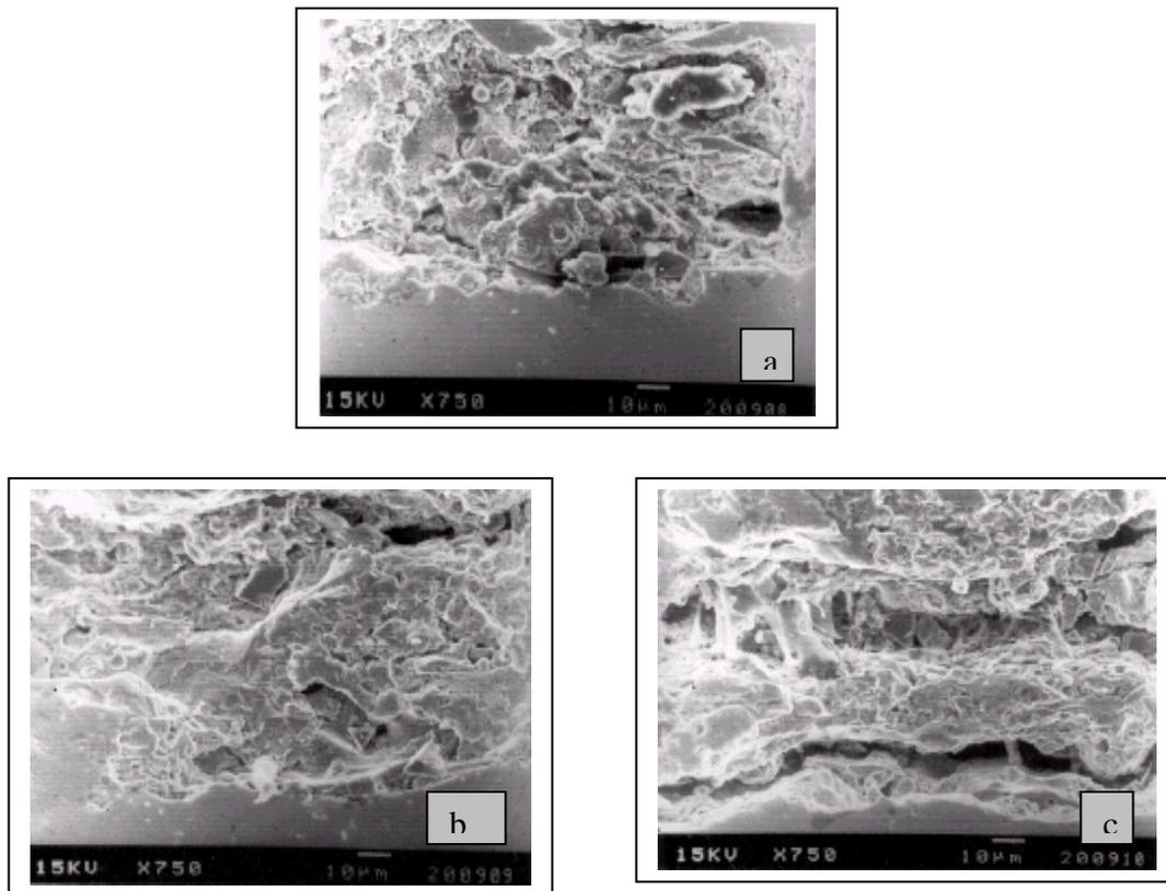
Figure 3 Interface microstructure of coatings made at 6, 9, 12 kW power levels
