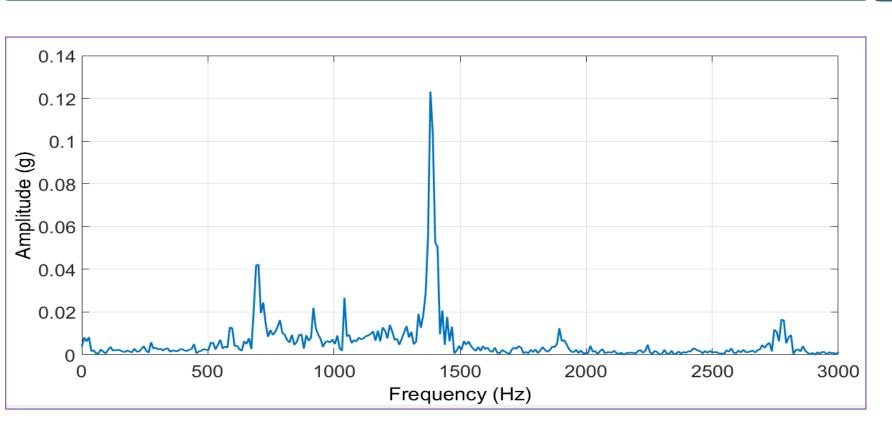
From the vibration signature, the level vibration is found to be significantly reduced near both the journal bearings.
