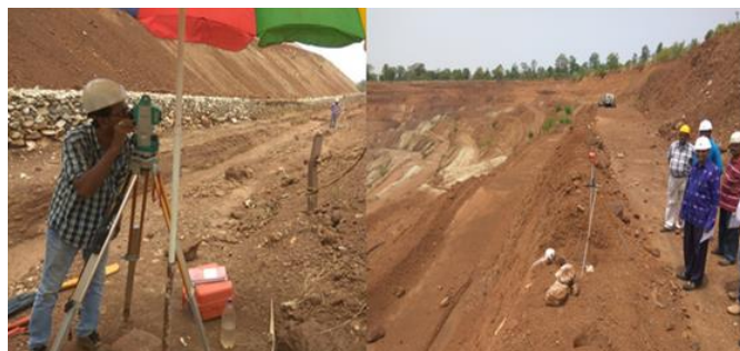
Fig 8: Monitoring of Dump slopes with total station at typical Chromite Mine
