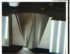
This injection mold was machined on a wire EDM using soft brass wire and tapering up to 30 degrees. The machine uses optional large-opening flush nozzles that prevent the wire from curling over the opening of the nozzle during the
