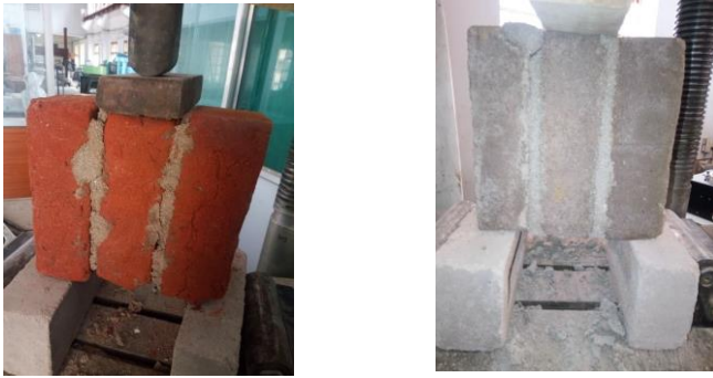
Fig. 2 Test set up for shear bond strength test with brick triplet specimens.
