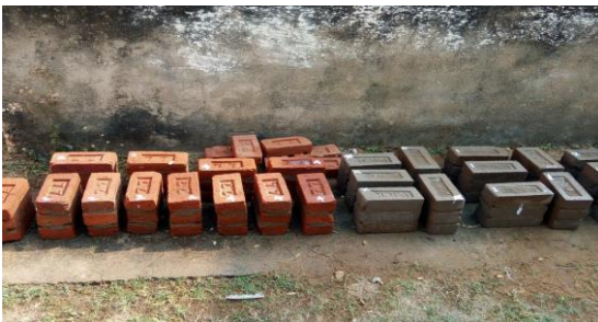
Fig. 1 Typical brick triplets for shear bond strength.
