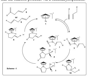
Scheme shown 1. as coordination of the alkyne and alkene by the coordinatively unsaturated ruthenium (+2) catalyst (1) to form complexes to form complexes (2) and (3), ruthenacyclopentenes (4) and (5) are possible, depending on the orientation of the alkyne. Although, in principle, the alkene can also opposite coordinate with the orientation (to generate
