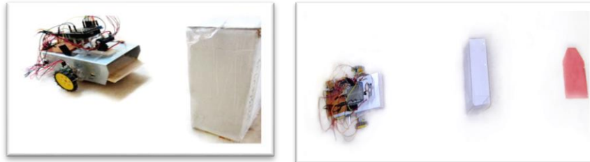
a) Developed differential mobile robot and b) its source, goal and obstacle in
