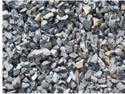
Fig. 5: Gravel (Natural Aggregates)
