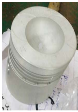
Fig. 4(b) Top view of the bowl in piston
