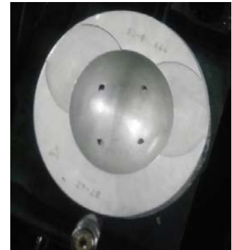
Fig. 5(b) Photographic view of internal jets
