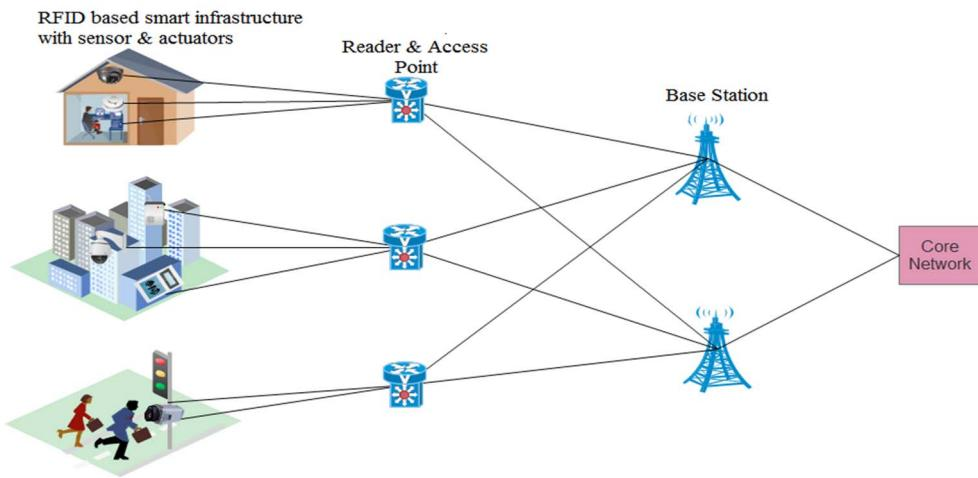
Fig.2. C-IoT network with its different functional units
