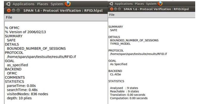
Fig.4. AVISPA result by the OFMC back-end and the CL-AtSe Back-end
