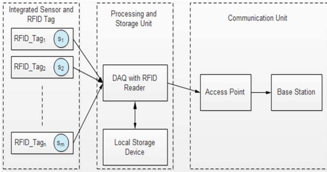
Fig.3. System block diagram for integrated-RFID communication process
