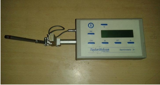
(a) Taylor/Hobson Surtronic 3+ surface roughness tester
