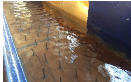
Figure 3: Arrangement of rigid rods as vegetation in experimental flume
