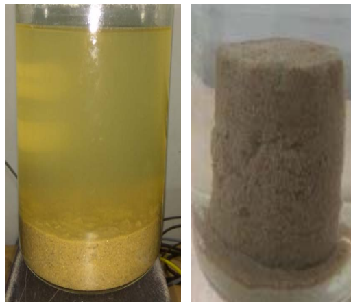
FIG.10. Dispersion test of Chilika sand with addition of biopolymer
