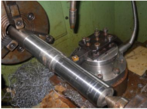
Fig. 3 Experimental set up for turning
