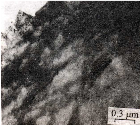
Fig. 7a - TEM of Quenched and tempered steel (450 °C, 1 hour) showing lath structure with dislocations
