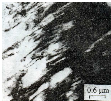
Fig. 8 - TEM of Quenched and tempered steel (600 °C, 1 hour) showing recovered structure
