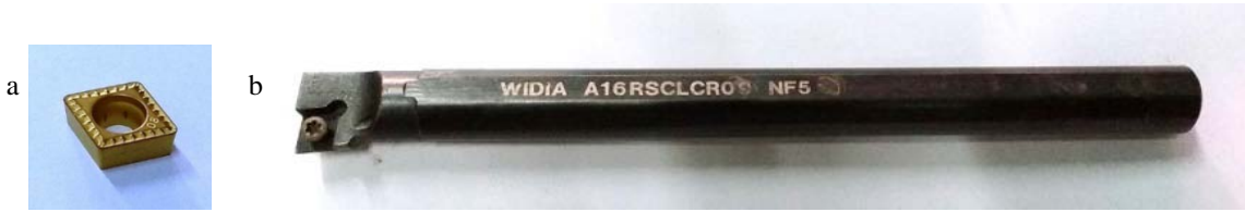
Fig. 1. (a) Cutting tool insert (CCMT-09T308-MU-TN2000); (b) Boring bar (A16R-SCLCR-09).
