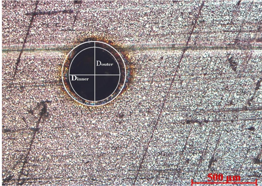
Fig. 2. Calculation of HAZ for laser drilling.
