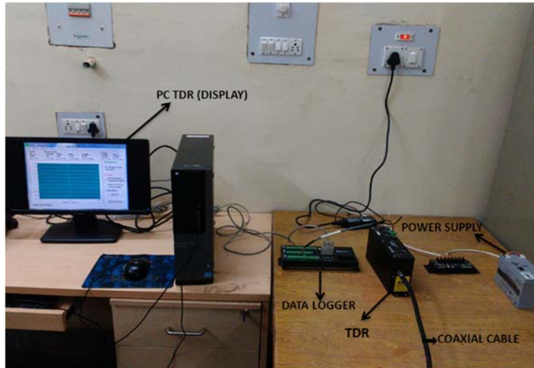
Fig.12 The lab set up including TDR.
