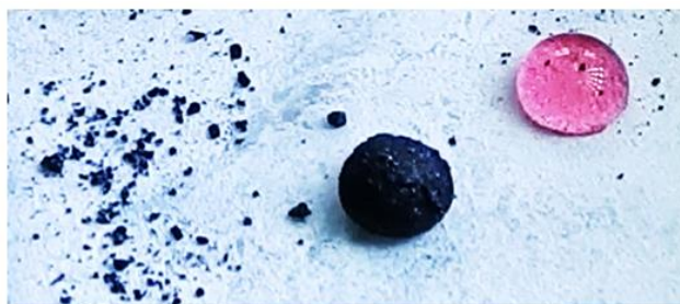
Fig. 3. Optical images of self-cleaning behavior of coating.
