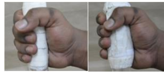
Fig. 1(b). Prototypes for handles of diameters 35 mm and 41 mm (left to right)
