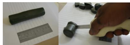
Fig. 5(b). Experimental task, a soft clay block (left) and a candidate cutting the clay block using knife having anatomically shaped handle
