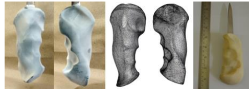
Fig. 4(b). Two different views of anatomically shaped handles over clay, corresponding digitized point cloud data and an ABS based 3D prototype with fitted blade (Left to right)
