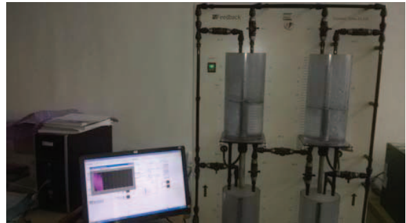
Fig. 6: Schematic of Experimental setup of coupled tank system
