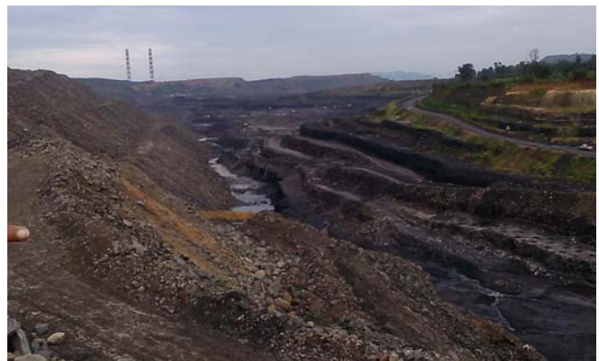
Fig. 3. A view of fly ash overburden admixture at dump site and working mine benches at JPL mines
