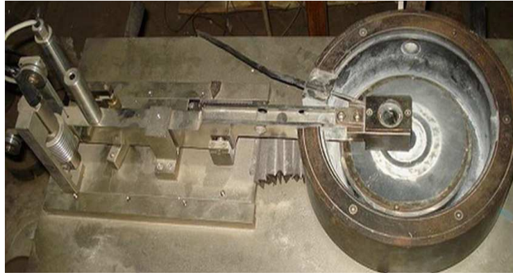
Figure 1: Pin on Disc Wear Test Machine
