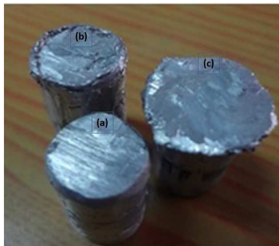
Figure 3: The Worn Surface of the Specimen (a) Al-Sample, (b) Al-Mg alloy and (c) Al-Mg-Si Composite
