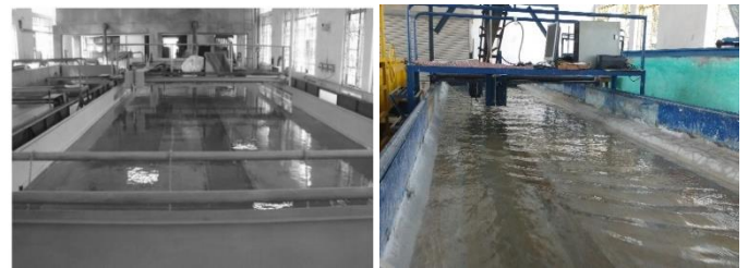
Figure 6. Photo of symmetric and asymmetric compound Channels fitted with instruments (NITR Series)
